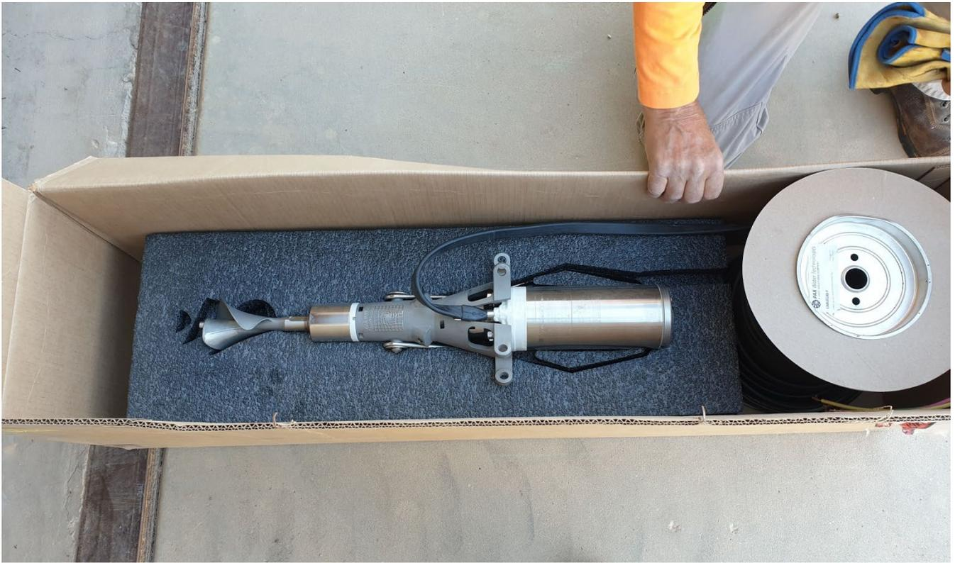
**New mechanical mixer unit was installed to replace the original faulty unit (#2). This replacement was performed under warranty.**
