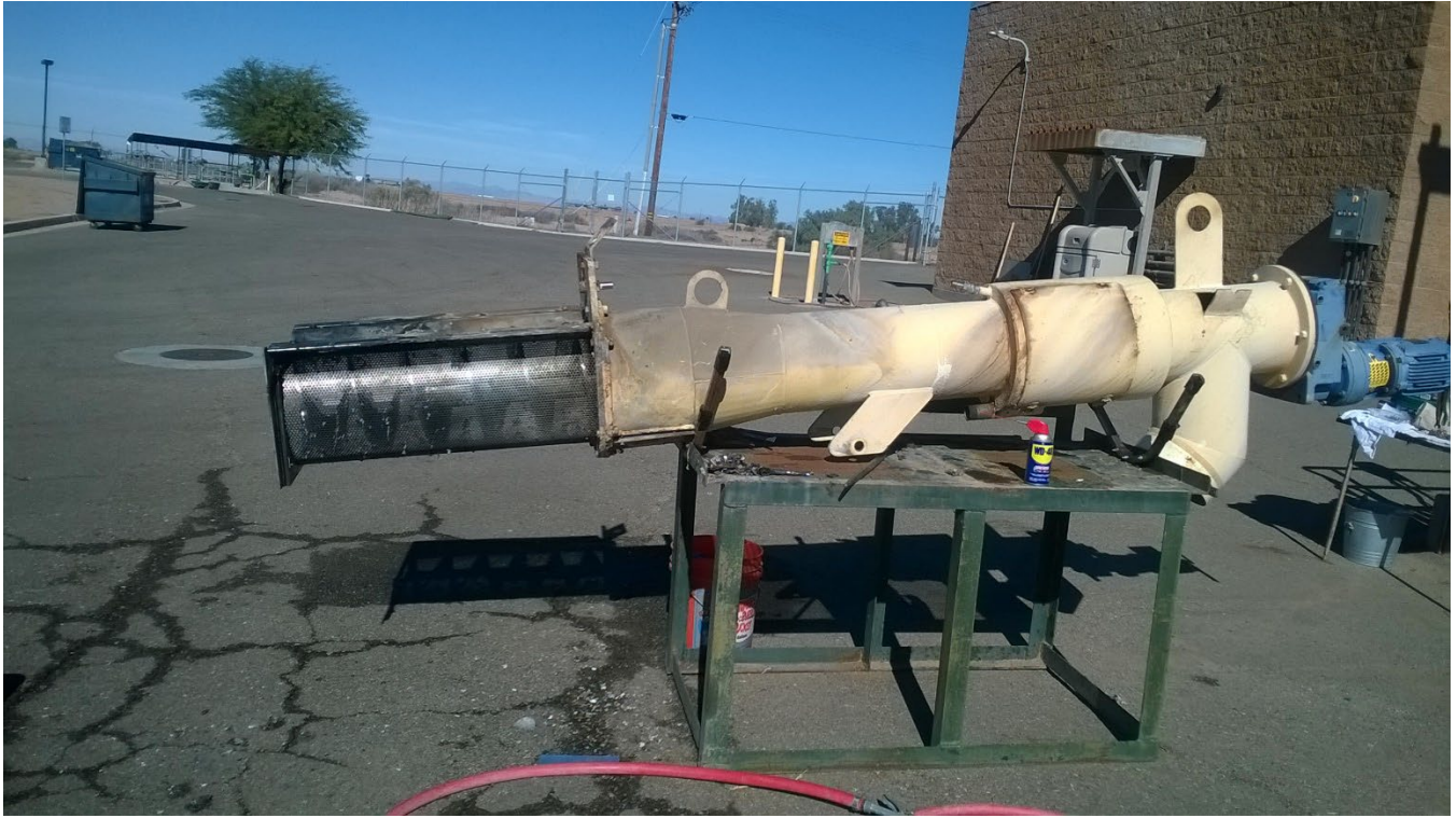
Side view of Raptor screening unit taken out of service for brush replacement
