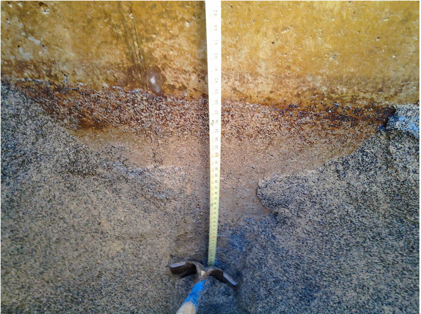
Measurement of filter media depth from top of bed to base of Filter cell #2.
