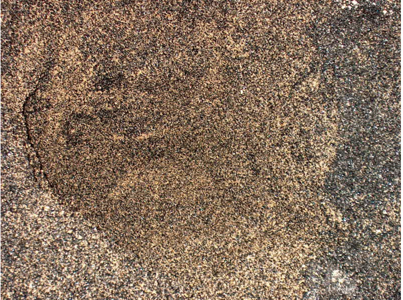
Close-up photo of #20 Silica sand media in Filter cell #3
