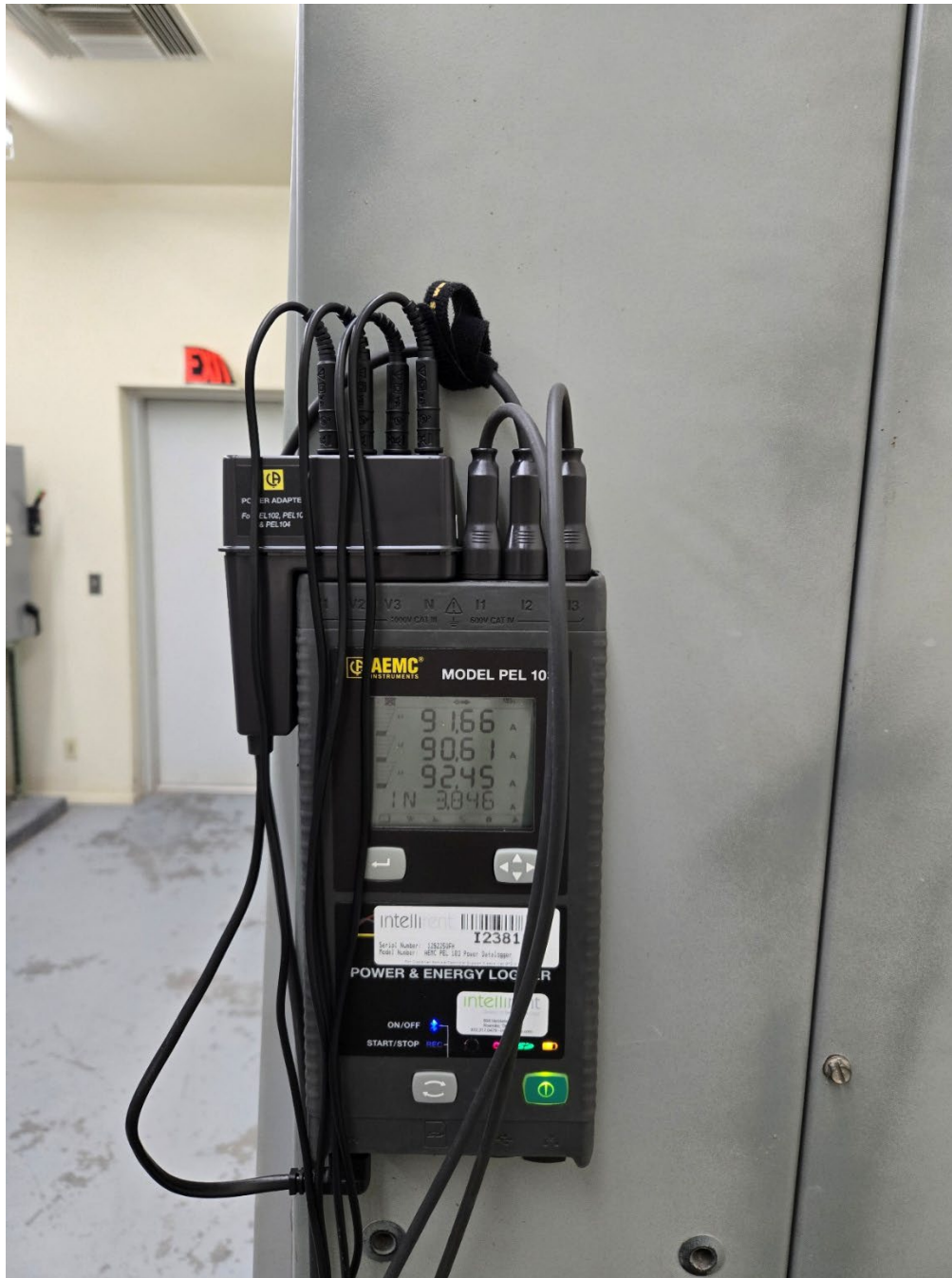
SiteLogiq continuous monitoring power usage recorder
